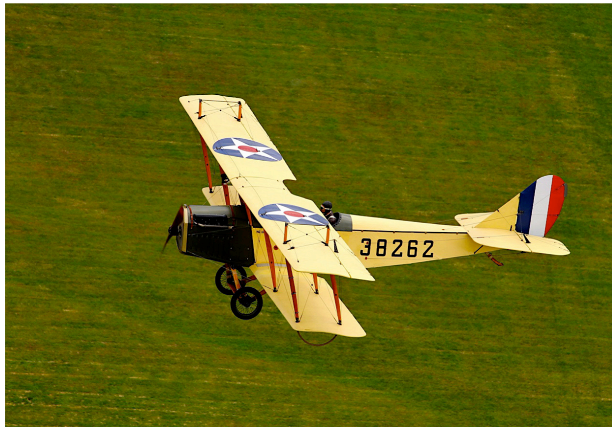
Left: The 5th Aviation School, and its successor 119th Aero Squadron flew the Curtiss JN-4 Jenny at Langley Field; the larger tail and modified wings cured the stability problems of the earlier JN-1. Far left: Just a month after America’s entry into World War I the government brought together leading engine builders to collaborate on the development of an advanced power plant, the result was the eight-cylinder Liberty engine; the first production engine is shown here next to future GEN “Hap” Arnold.
