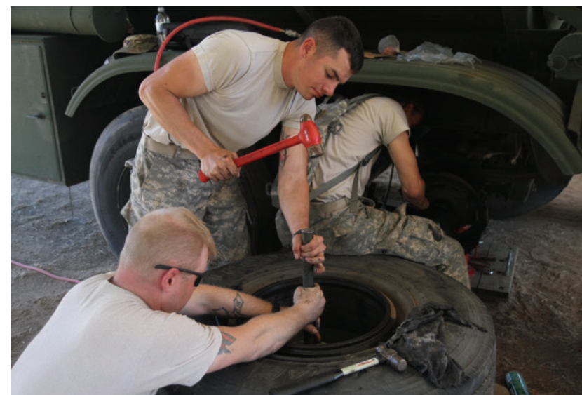
Soldiers from the 561st Regional Support Group conduct maintenance of tankers during the Quartermaster Liquid Logistics Exercise (QLLEX), June 15, 2016. Pvt. 1st Class Tyler Giammasi, of Wichita, Kan., works to fix a blown tire seal on a tanker.
