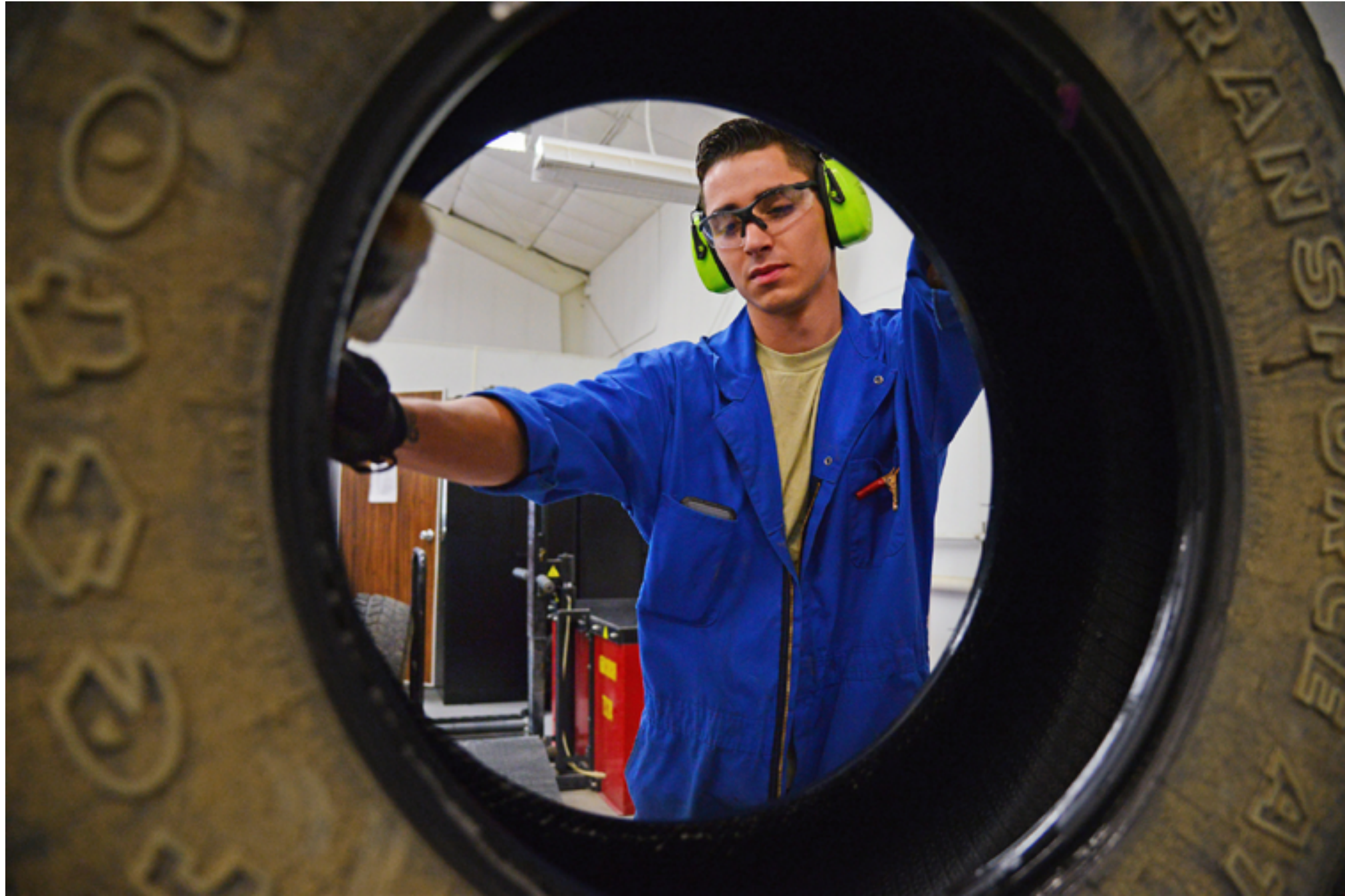
Senior Airman Brennan Popp, 341st Logistics Readiness Squadron mission generating vehicular equipment maintenance technician, lubricates the inside of a tire July 7, 2016, at Malmstrom Air Force Base, Mont. The lubrication helps the tire fit over a rim when a new tire is mounted. (U.S. Air Force photo/Airman 1st Class Daniel Brosam)
