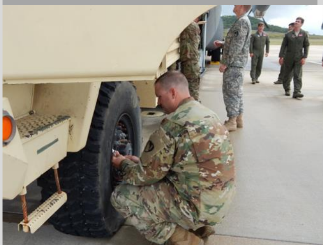
MAJ Jones releasing air from tires in order to facilitate vehicle loading
