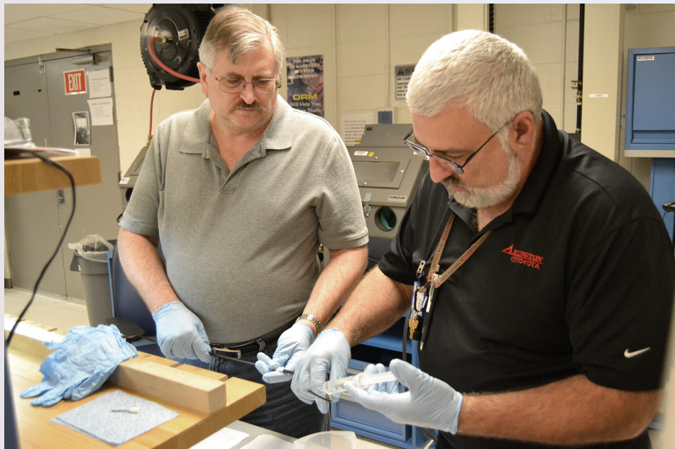
Artisans Jim Calhoun, left, and Stephen Frankewicz, right, apply epoxy to a sample cable before they test its strength at Hangar 1000. The cable is part of the reeling machine that lowers the sonar into the water.
