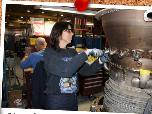
Aircraft Engine Mechanic Susan Fiest removes cables from fuel nozzles on an F414 engine
