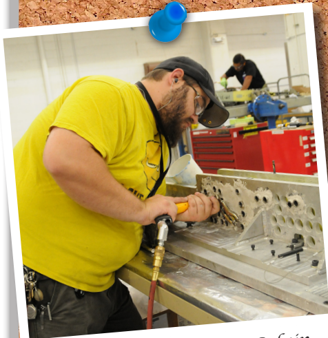
Sheet Metal Mechanic Calvin Tapley drills on an F/A-18 missile rib in the FRCSE wing shop
