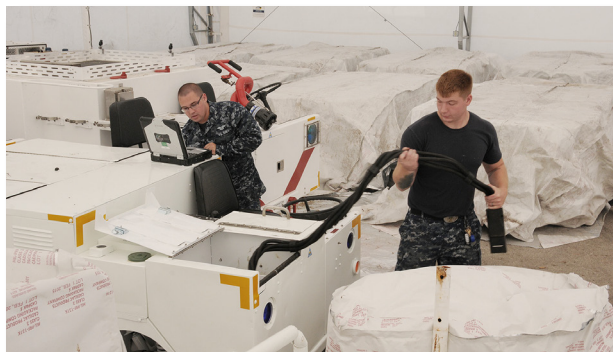
Aviation Support Equipment Technician (AS) Airman (AW) Shane McMaster, left, and AS3 Travis Shelhamer, right, of USS Iwo Jima's 900 Division, perform maintenance on a mobile electric power plant in a shelter built for the ship's equipment at FRCSE Detachment Mayport. The vehicle is used to supply power to aircraft aboard the ship.
