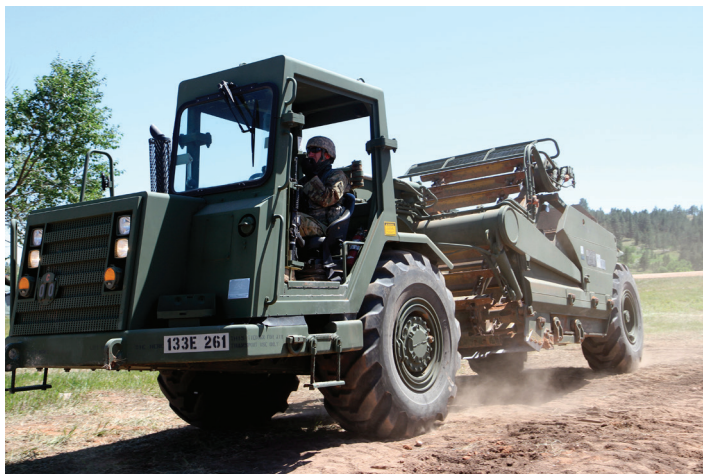
U.S. Army Spc. Ian Staley, heavy equipment operator with the 133rd Engineer Company of the Wyoming National Guard, operates a scraper to prepare the road site for further construction. (U.S. Army National Guard photo by Spc. Kristin Lichius)
