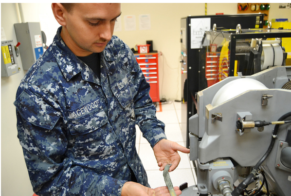
AT2 Cody Hagewood shows some corrosion on a grounding strap for the reeling machine that military depot Sailors and artisans will repair.
