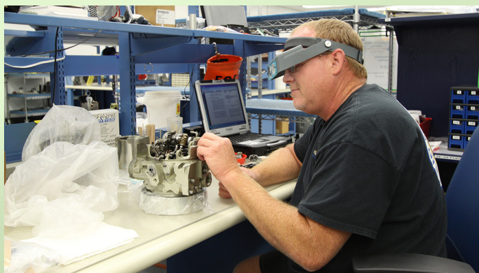
C.J. Carroll, a pneudraulics systems mechanic at Fleet Readiness Center Southeast Fuel and Accessories Facility, reassembles a fuel control system for a TF-34 engine.
