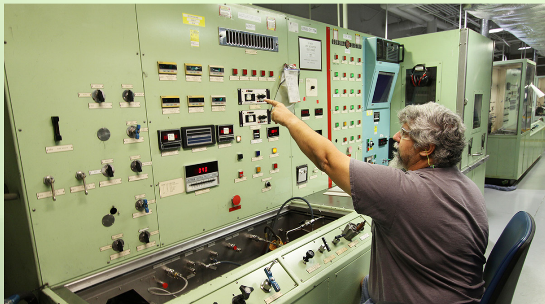
Pneudraulics mechanic Charles Kresol fine-tunes the settings on an F-404 Actuator Test Stand at FRCSE's Fuel and Accessories Facility.
