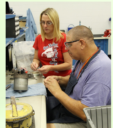
Pneudraulics systems mechanics Steve Thomas, right, and Laura Smith examine an air filter for a T-34 engine at the FRCSE Fuel and Accessories Facility.
