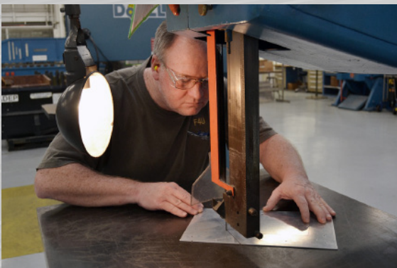
Aircraft Tooling Maker Dale Holt cuts off the excess aluminum from a chem-milled part in the layout and manufacturing shop Nov. 16. After it is sanded, pre-treated and primed, the part will be ready to return to the fleet.
