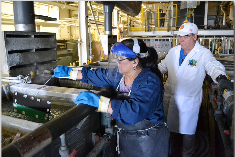
Electroplater Marissa DeMent lowers a part into a rinsing solution after it comes out of the chemical milling solution as Engineer Technician Rodney Williamson looks on. The upper half of the panel has been chemically milled.
