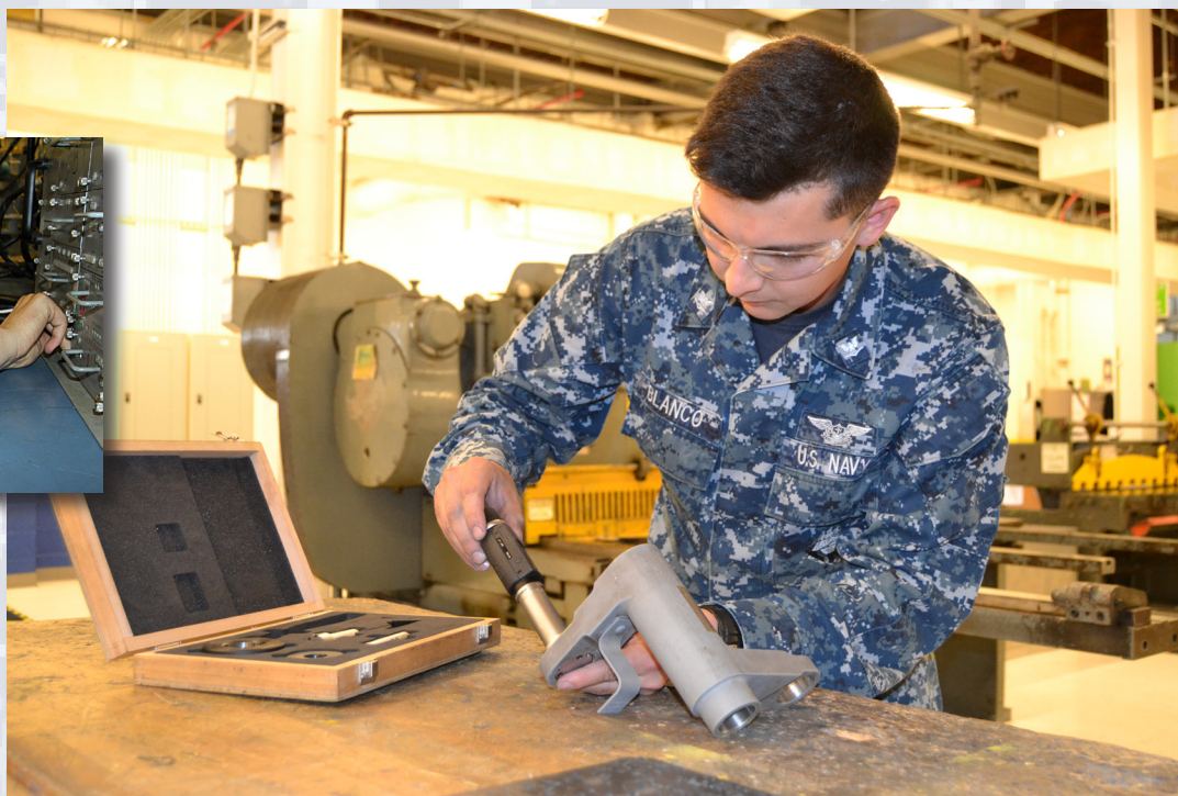
AM3 Rane Blanco measures the bore on an aviation component at FRCSE Det Jacksonville April 30.
