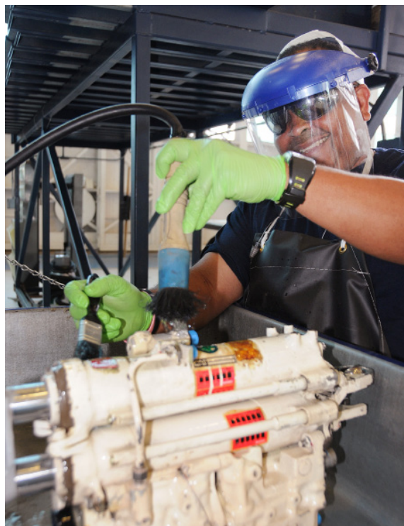
Godfrey McDowell, an F/A-18 aircraft mechanic, uses a solvent tank to clean a trailing-edge flap actuator to prepare it for inspection April 15. McDowell is one of many FRCSE artisans who make suggestions to mitigate unsafe practices. FRCSE leadership encourages all employees to take part in the safety program. This is one of the many initiatives that led the command to earning the CNO's 2014 Safety Excellence Unit Award for medium industrial, shore activity.
