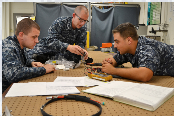
Sailors test the continuity of a cable in the repair shop at FRCSE Detachment Jacksonville. More than 600 Sailors assigned to the detachment played a role in the command's performance in a recent aviation maintenance inspection.
