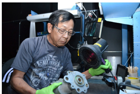
Rafael Sur, an inspector with the NDI shop, uses a black light to examine an aviation component for cracks and defects.
