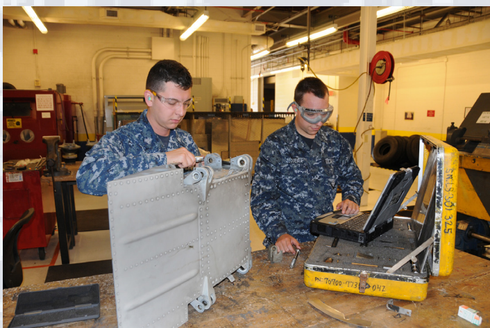
AMAN Nicholas Zequeira (right) provides a process check to AM3 Rane Blanco who is using a micrometer to measure lug and washer bores on an H-60 center stabilizer at FRCSE Detachment Jacksonville.
