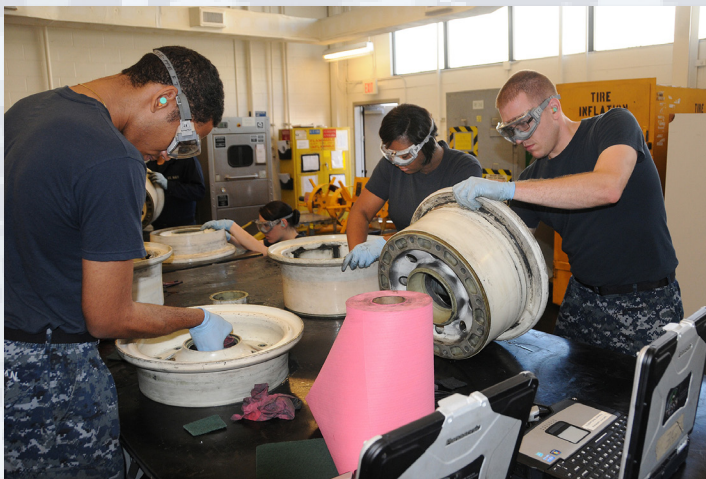
(From left) AMAA Frederick Dunstan, AMAN Nykie Carr (kneeling), AM3 Shakita Howard, and AM2 Gregory Anderson clean disassembled P-3 Orion rims at FRCSE Detachment Jacksonville's Tire Shop. 'Tire and Wheel' was one of 41 aviation maintenance programs inspected during the detachment's recent aviation maintenance inspection (AMI). Forty programs received "on-track" ratings during the inspection.
