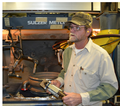
Plasma Spray Shop Work Lead Mike Allen holds a metal part he and co-worker Brian Veek built to use on the 6P thermal spray gun. The spray gun is used to apply a protective metal coating on aircraft engine casings.
