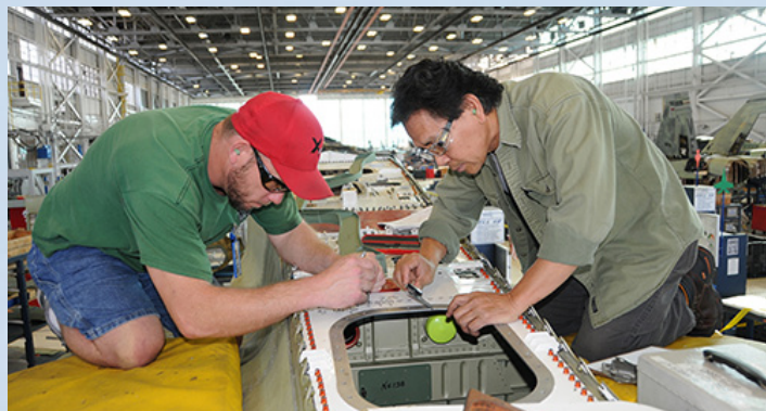
Machinists Lonnie Conditt, left, and Narom Orr measure holes to ensure alignment of an F/A-18 part on the production line.
