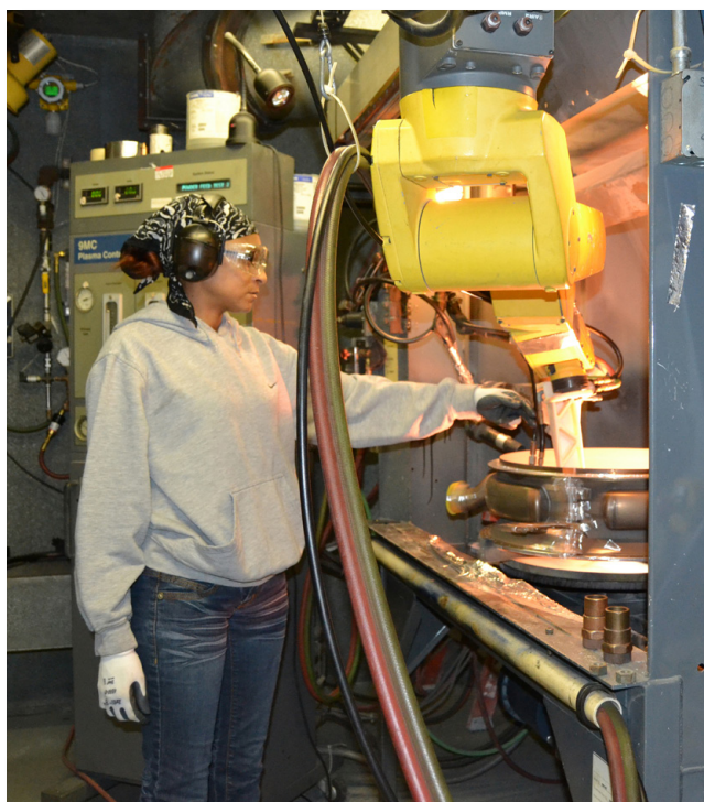
Milena Carter checks the hoses on a 6P thermal plasma spray gun while using a heated spraying technique to apply a thin metal powder coating on engine casings in the plasma spray shop.
