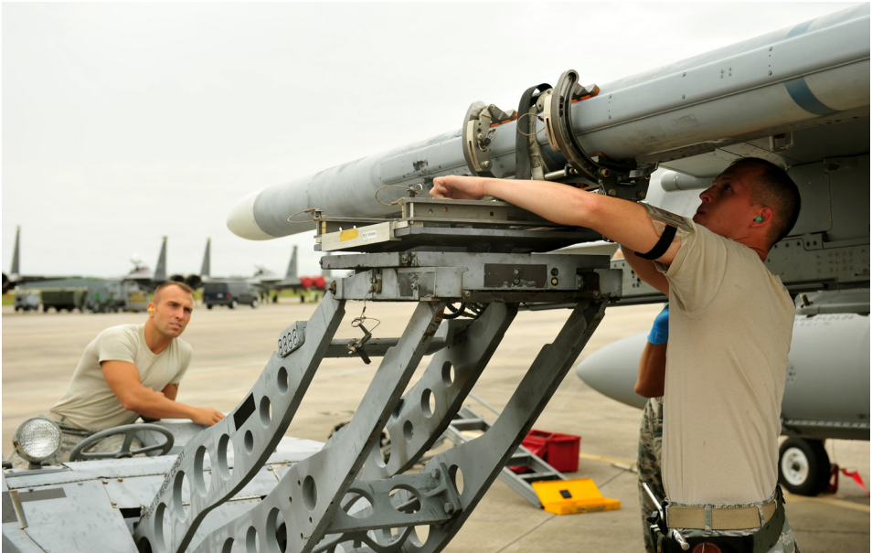
Senior Airman Jake Sorosiak and Staff Sgt. Samuel Kimple, weapons loaders from the 180th Fighter Wing, upload an Air Intercept Missile, commonly referred to as an AIM-120, to be loaded on an F-16 Fighting Falcon Sept. 15, 2015 at Tyndall Air Force Base, Florida.
