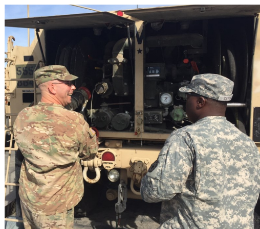
SPC Miller and SPC Taylor prepare for fueling by recirculating the fuel through the fuel truck.
