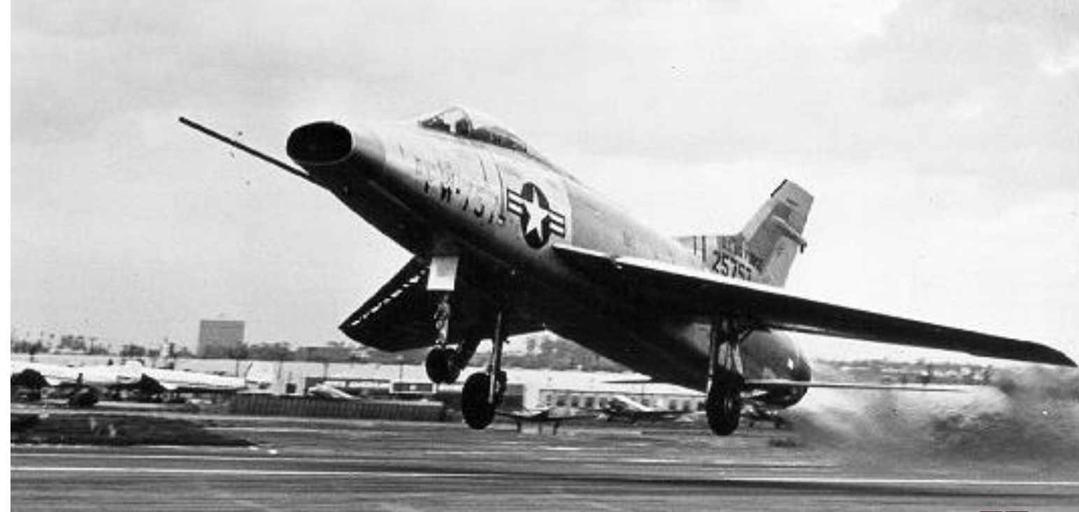
An early production of the F-100A (note the short tail) leaps into the air from a Los Angeles airport runway. North American's Inglewood factory was located on the eastern edge of the airport. (USAF photo)
