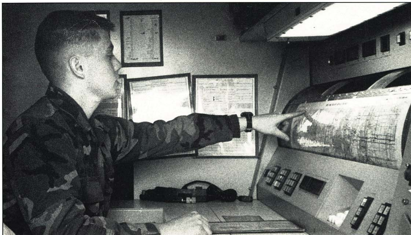
Spc. Leroy T. Peoples uses the Q36 computerized radar system to help pinpoint targets for artillery gunners.
