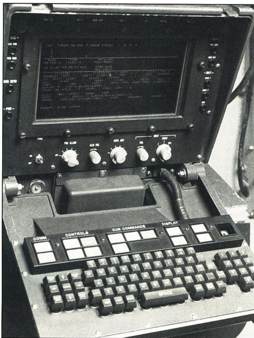
The Battle Computer System coordinates data from forward observers and from the radar and meteorological sections.
