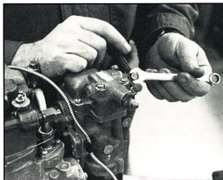
Sgt. 1st Class Craig Bonnell performs maintenance on the AH-1 fuel system.
