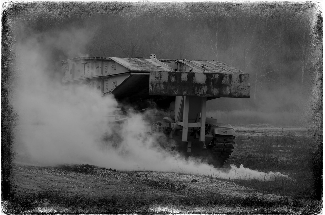
An armored vehicle-launched bridge is moved into position during a gap-crossing operation. (Photo by Ms. Dawn Arden, Fort Leonard Wood Guidon .)
