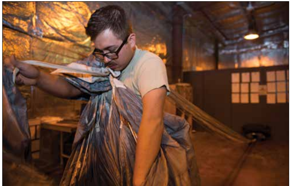
LEFT: Senior Airman Mike Garcia, 82nd Expeditionary Rescue Squadron aircrew flight equipment rigger, secures the suspension lines onto the outside of a parachute using rubber bands, Camp Lemonnier, Djibouti, March 26. The correct tolerances must be maintained to ensure proper operation. RIGHT: Senior Airman Dwain Miller, 82nd Expeditionary Rescue Squadron aircrew Flight Equipment rigger, carefully stacks the folds of a parachute during packing, at Camp Lemonnier, Djibouti, March 26. Photos by Staff Sgt. Carlin Leslie
