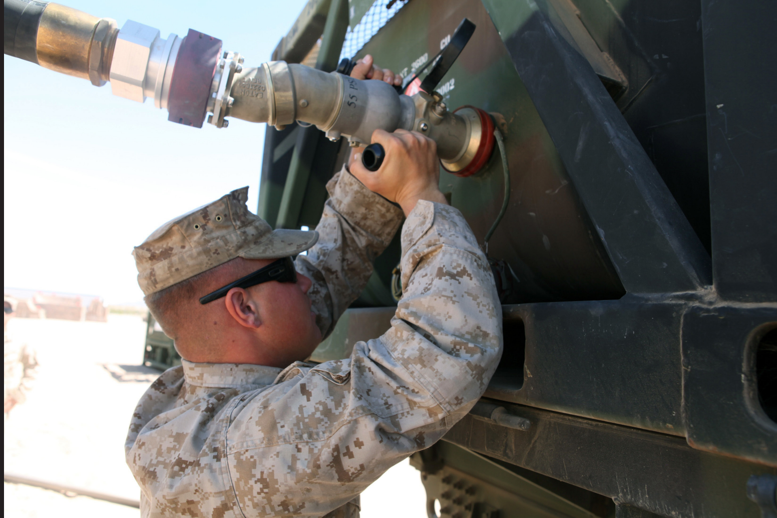
Top left: Private First Class Brenen Tischner, left, a Motor Transportation Operator, with 1st Transport Support Battalion, Combat Logistics Regiment 1, 1st Marine Logistics Group, attaches a fuel hose to an AMK-23 Medium Tactical Vehicle Replacement with the help of two other Marines during routine refueling maintenance on the outskirts of Marine Corps Air Station Yuma, Ariz., April 10, 2015.
