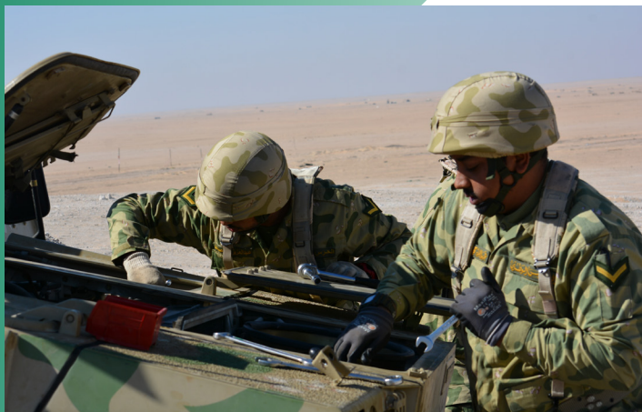
Two lance corporals in the Kuwait National Guard remove some bolts to take a fan out of the Panhard vehicle out and replace it at Udairi Range Training site in Kuwait, Jan. 21.
