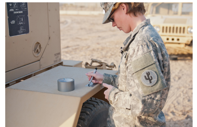
Sgt. Breanna Carder, a cargo specialist serving as part of the Arrival/Departure Air Cargo Group in Kuwait, places tape on a generator at its axles as part of gathering the center weight and axle balance for documentation purposes prior to Air Force movement.
