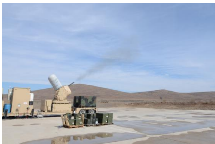
A Land-based Phalanx Weapons System engages an indirect fire target on Fort Sill, Oklahoma during an indirect fires protection capability unit conversion validation exercise on February 20, 2015. The weapon system fires a self-detonating 20mm round to intercept indirect fire threats. (U.S. Army photo by Capt. Corey Robertson, 31st ADA BDE PAO / Released)
