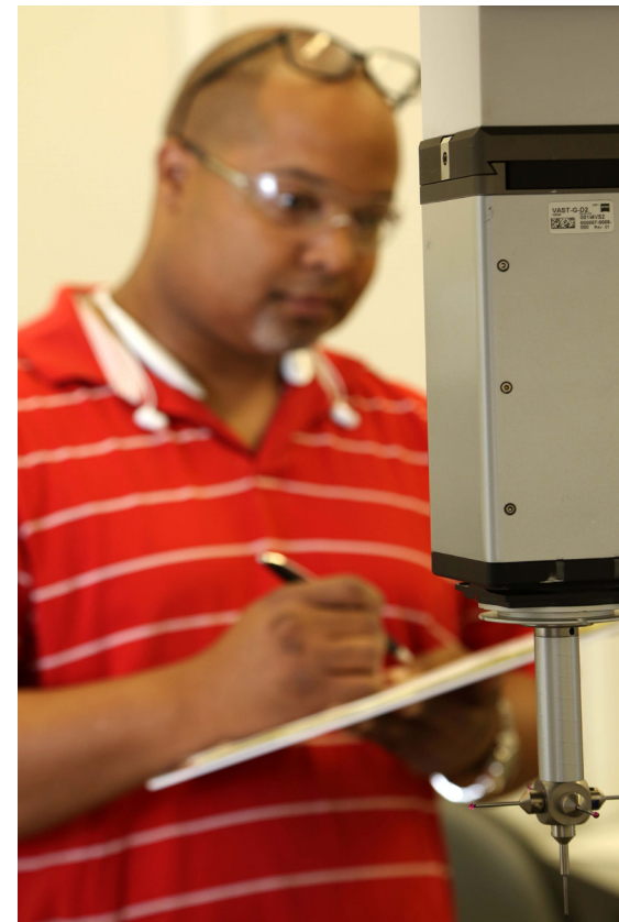
Marlow Bass, Sr., a Defense Contract Management Agency Lockheed Martin Dallas Keystone quality assurance specialist, ensures a coordinate measuring machine correctly measures a component so that it meets the tolerances of the drawing. (DCMA photos by Thomas Perry)
