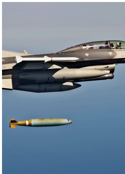
An inert Mark-84 bomb is released from a BRU-61 carriage system equipped F-16 during a test over the Gulf of Mexico. (Air Force photo by Staff Sgt. Joely Santiago)
