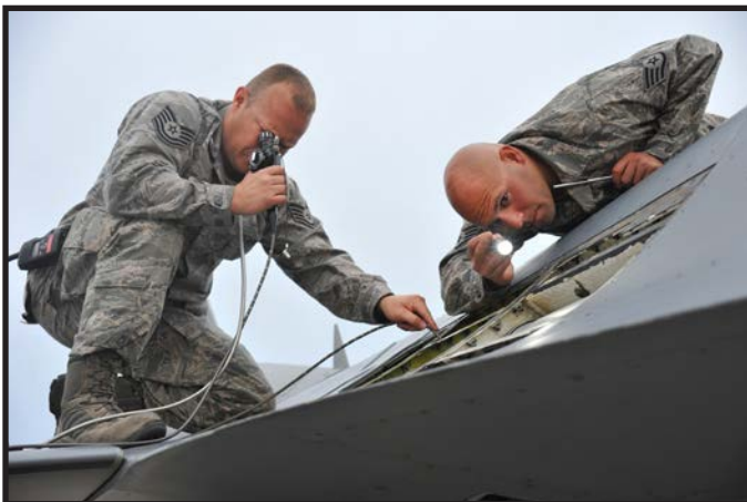
U.S. Air Force Tech. Sgt. Dan Sohnrey, an engine mechanic with the 180th Fighter Wing, uses a borescope to inspect the inside an F-16 Fighting Falcon with the assistance of crew chief, Staff Sgt. Michael Woronec, at the Alpena Combat Readiness Training Center in Alpena, Michigan, Aug. 21, 2014. The 180th Fighter Wing deployed to the CRTC to participate Operation Northern Strike, a joint exercise led by the National Guard that demonstrates the combined power of the air and ground forces. (Air National Guard photo by Staff Sgt. Amber Williams/Released)
