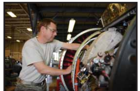
Staff Sgt. Randall Roelker changes a T5 Amplifier on a TF34-100A Turbo Fan Engine that is used on the A-10C.
