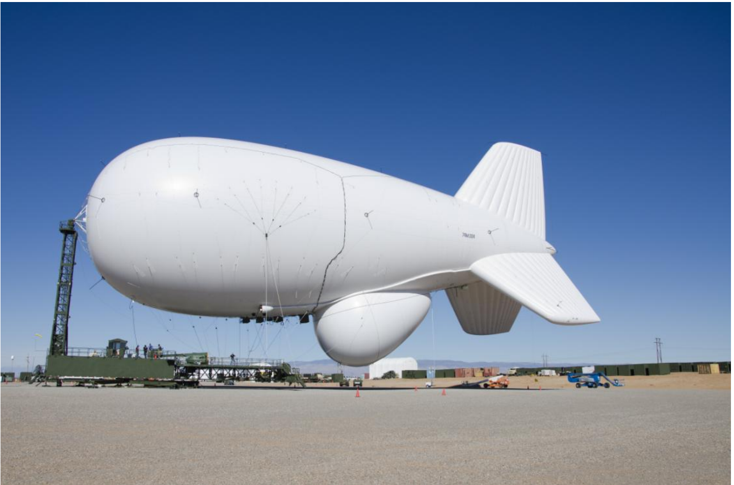
A Joint Land Attack Cruise Missile Defense Elevated Netted Sensor System, or JLENS, aerostat is readied for launch near Orogrande gate at White Sands Missile Range, N.M. in this April, 2012 file photo. A single JLENS aerostat can carry a surveillance radar or fire control radar up to 10,000 feet allowing the radar to see over surrounding terrain.
