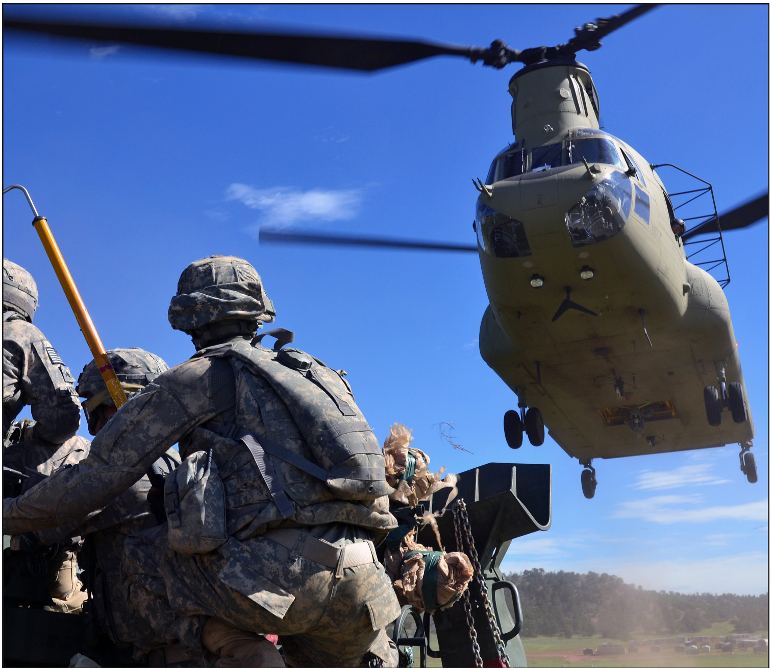
Soldiers from 2-12th Field Artillery Company hook a M777A2 Howitzer to a CH-47 Chinook from 2nd General Support Aviation Battalion, 4th Aviation Regiment, 4th Combat Aviation Brigade, 4th Infantry Division, during elevation sling-load training exercise on Fort Carson, Colo.
