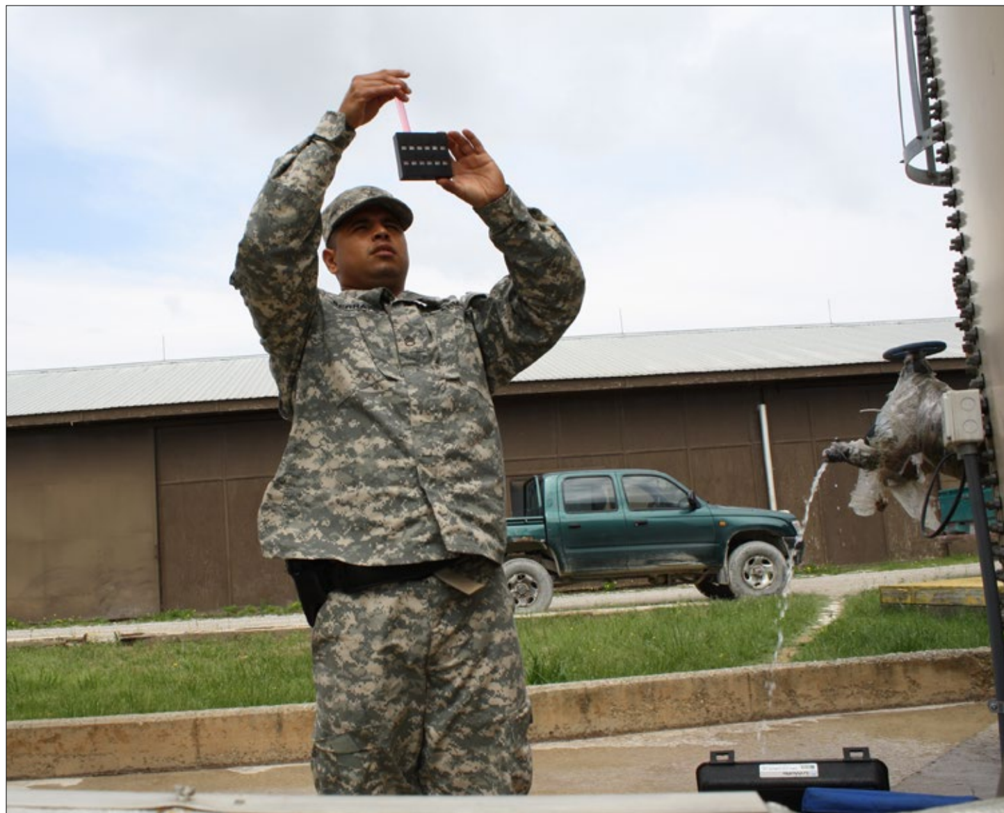
Staff Sgt. Erik D. Serrato, TF Med preventive medicine noncommissioned officer conducting chlorine and PH levels of Camp Bondsteel water, Kosovo, July 22. Camp Bondsteel water treatment plant produces 1.13 million liters of water per day.
