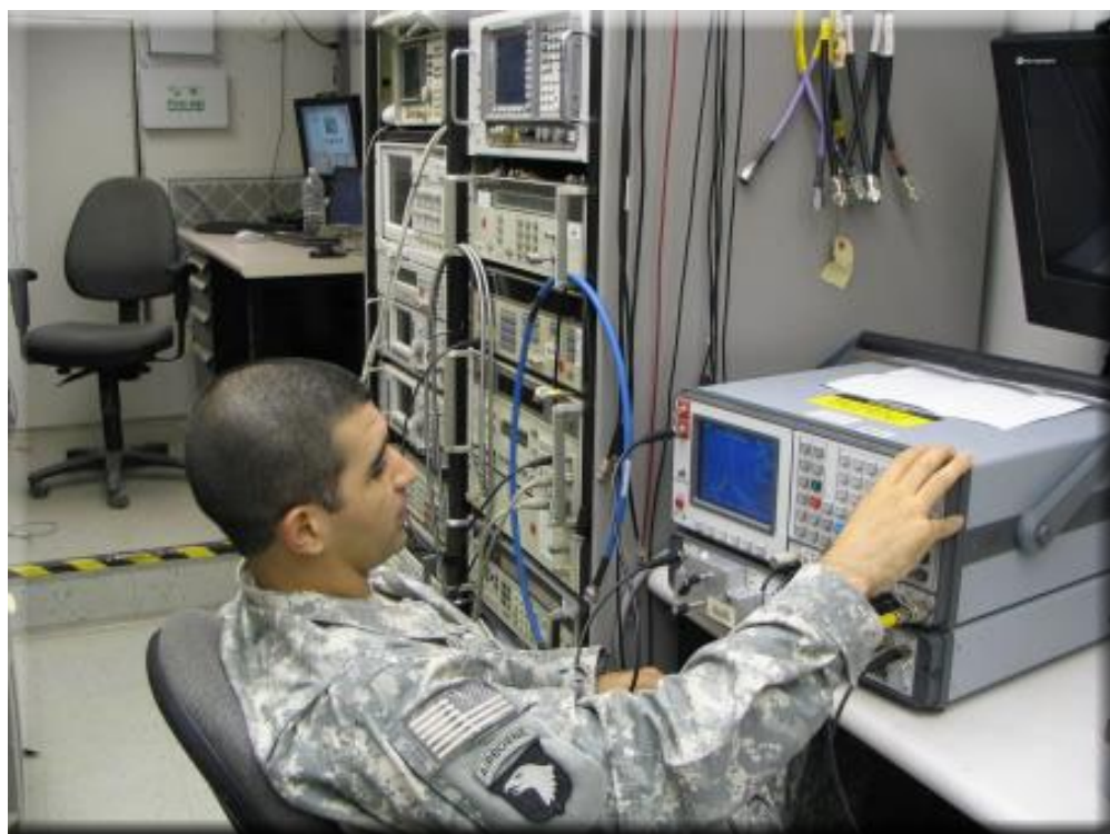
Cpl. Yilian Lu, a test, measurement, and diagnostic equipment shop foreman assigned to the 514th Support Maintenance Company, troubleshoots and repairs an EEDM503B multimeter.
