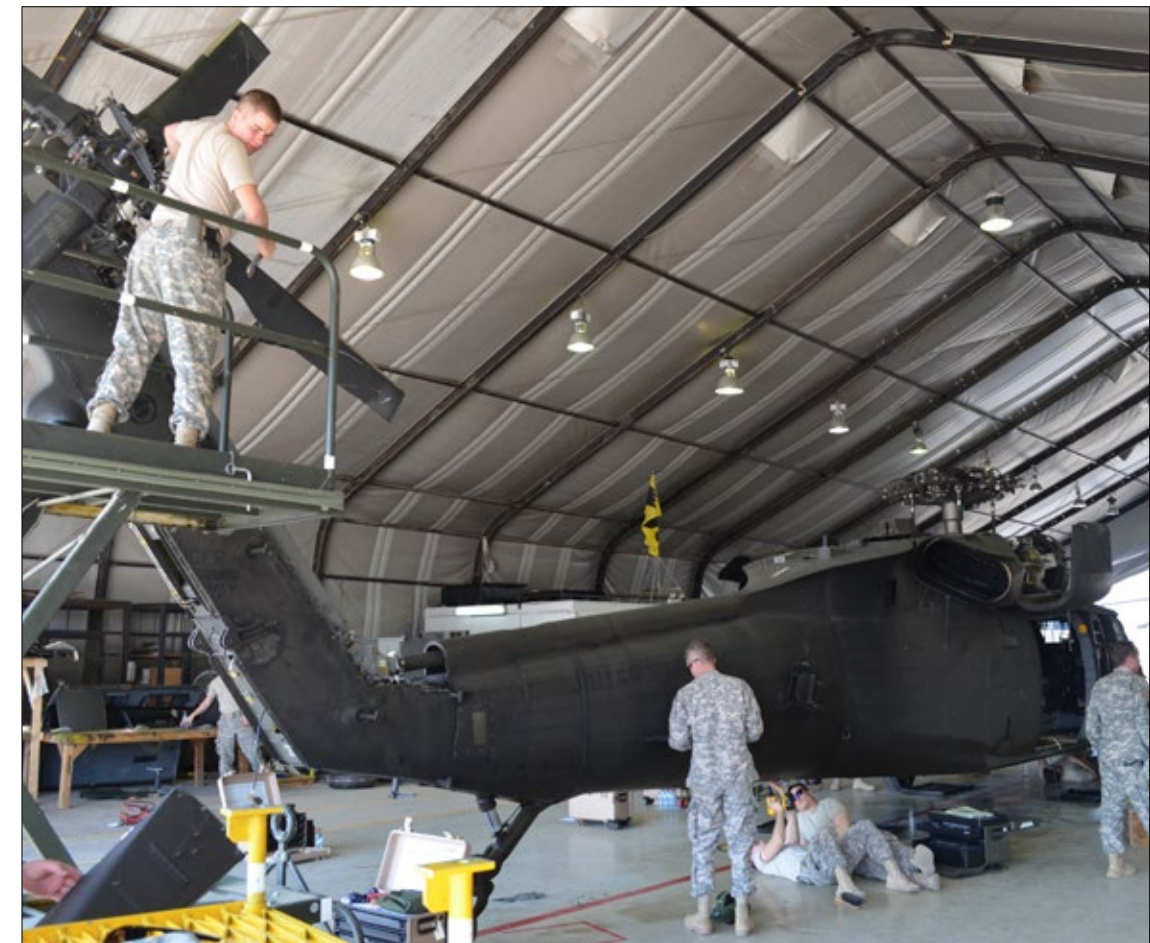
Soldiers with B Company, 248th Aviation Support Battalion, Iowa Army National Guard, conduct removal of components and conduct inspections while performing a Phase Maintenance Inspection I on a UH-60 Black Hawk helicopter, July 8. (Courtesy photo)
