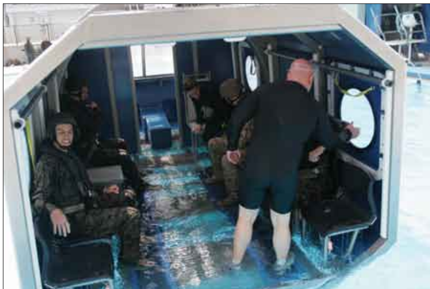
The modular amphibious egress trainer, commonly called the "helo dunker," can simulate the interior of a CH-46 or CH-53 helicopter.
