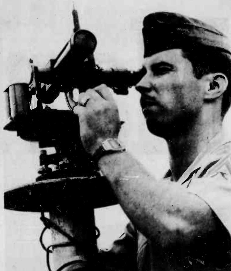
TRACKING — Corporal Mike Beaudette, azimuth and elevation of the balloon. The Station Weather Service, tracks an ascending weather balloon with the aid of a theodolite. The instrument records the readings are then compared to a chart that shows the rate of ascent.
