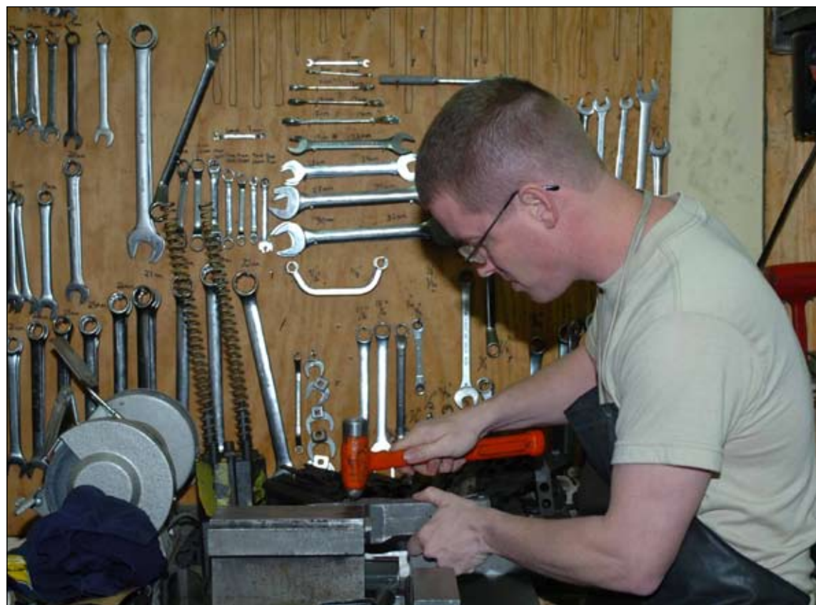
Sgt. Todd G. Kerwin, small arms repairman with the 758th Maintenance Company from Conway, Ark., tightens the rivet arms of the buffer housing. The rivets are designed only to only move up and down, not left and right.
