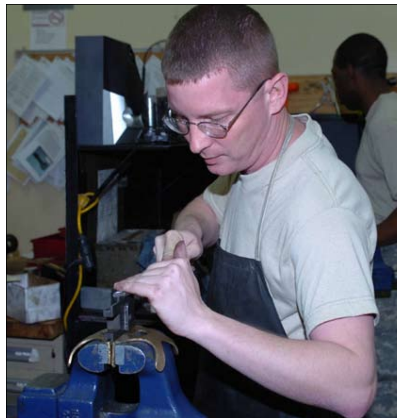
(Left) Spc. Eric J. Rose, small arms repairman with the 758th Maintenance Company from North Richland Hills, Texas, tightens the lacing wire on a .50 caliber machine gun in order to make sure the screws will not loosen up. (Right) Sgt. Todd G. Kerwin, small arms repairman with the 758th Maintenance Company from Conway, Ark., grinds a metal plate in order to smooth out its edges.
