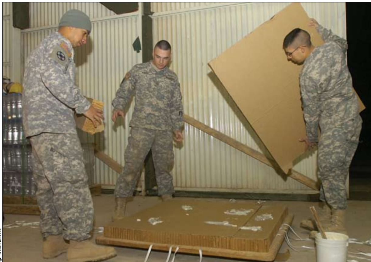
Sgt. 1st Class Mark Bell Staff Sgt. Franz Tovar, Spc. James Ahern and Spc. Wesley Desouza, all assigned to the 600th Quartermaster Detachment (Airborne), based at Fort Bragg, N.C., glue together Energy Dissipation Material that provides protection and absorbs the energy of an airdrop for the bottom of the Improved Cargo Delivery System.
