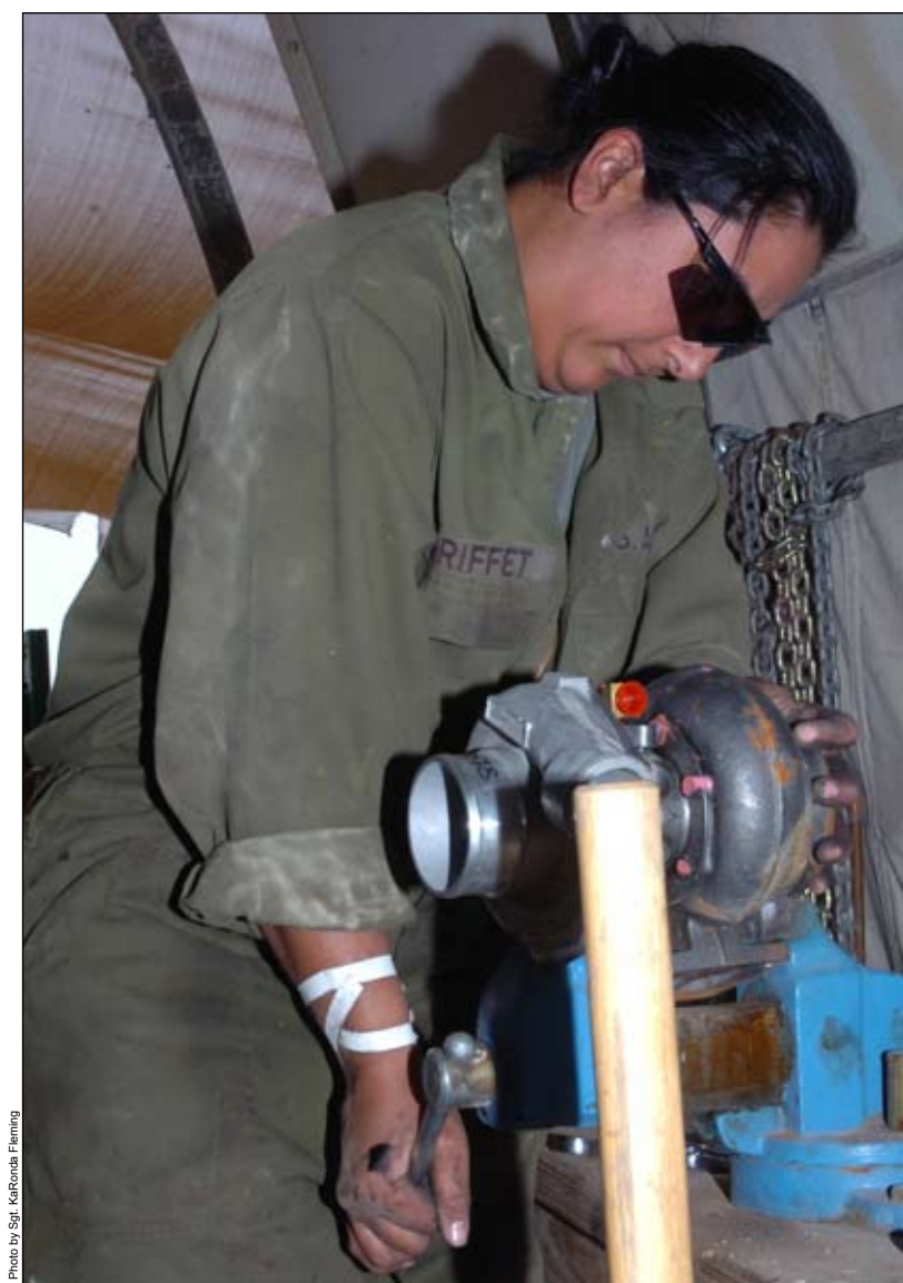
Spc. Veronica C. Gutierrez with the Headquarters and Support Company, 449th Aviation Support Battalion, loosens the bolt on a turbo charger that was recently taken out of a generator.
