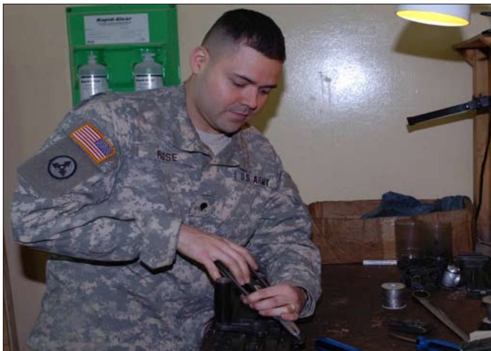
(Left) Spc. Eric J. Rose, small arms repairman with the 758th Maintenance Company from North Richland Hills, Texas, tightens the lacing wire on a .50 caliber machine gun in order to make sure the screws will not loosen up. (Right) Sgt. Todd G. Kerwin, small arms repairman with the 758th Maintenance Company from Conway, Ark., grinds a metal plate in order to smooth out its edges.
