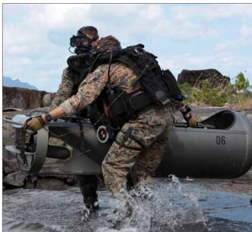
Cpl. Peter E. Kober, left, and Sgt. Scott A. Hulsizer carry their diver propulsion device into the water to begin their dive Jan. 22, during a certification course at Marine Corps Base Kaneohe Bay, Hawaii. The DPD is a battery-powered vehicle capable of carrying two divers and their equipment while submersed out of sight. The course was a part of Exercise Sandfisher 2014. Kober and Hulsizer are reconnaissance men with Company B, 3rd Reconnaissance Battalion, 3rd Marine Division, III Marine Expeditionary Force. Photo by Cpl. Brandon Suhr
