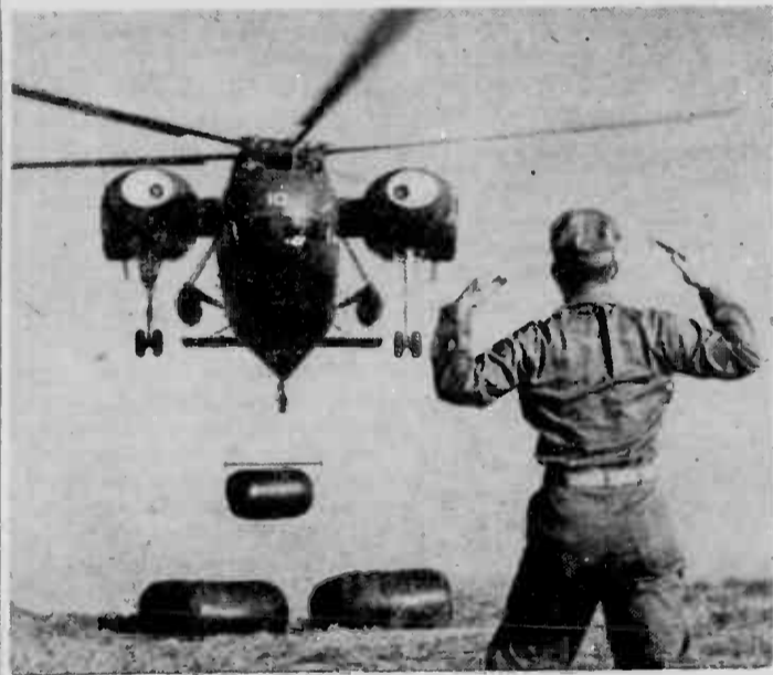
CROSS-EYED BUG — This Marine HR2S-1 helicopter gives the appearance of being a giant, cross-eyed bug laying an oblong egg, but is demonstrating its versatility by gingerly lowering a rubber fuel tank containing 525 gallons of gasoline. The HR2S-1 is one of three types of helicopters scheduled to participate in operation CLEAR RIDGE. Photo by 1stMarDiv.
