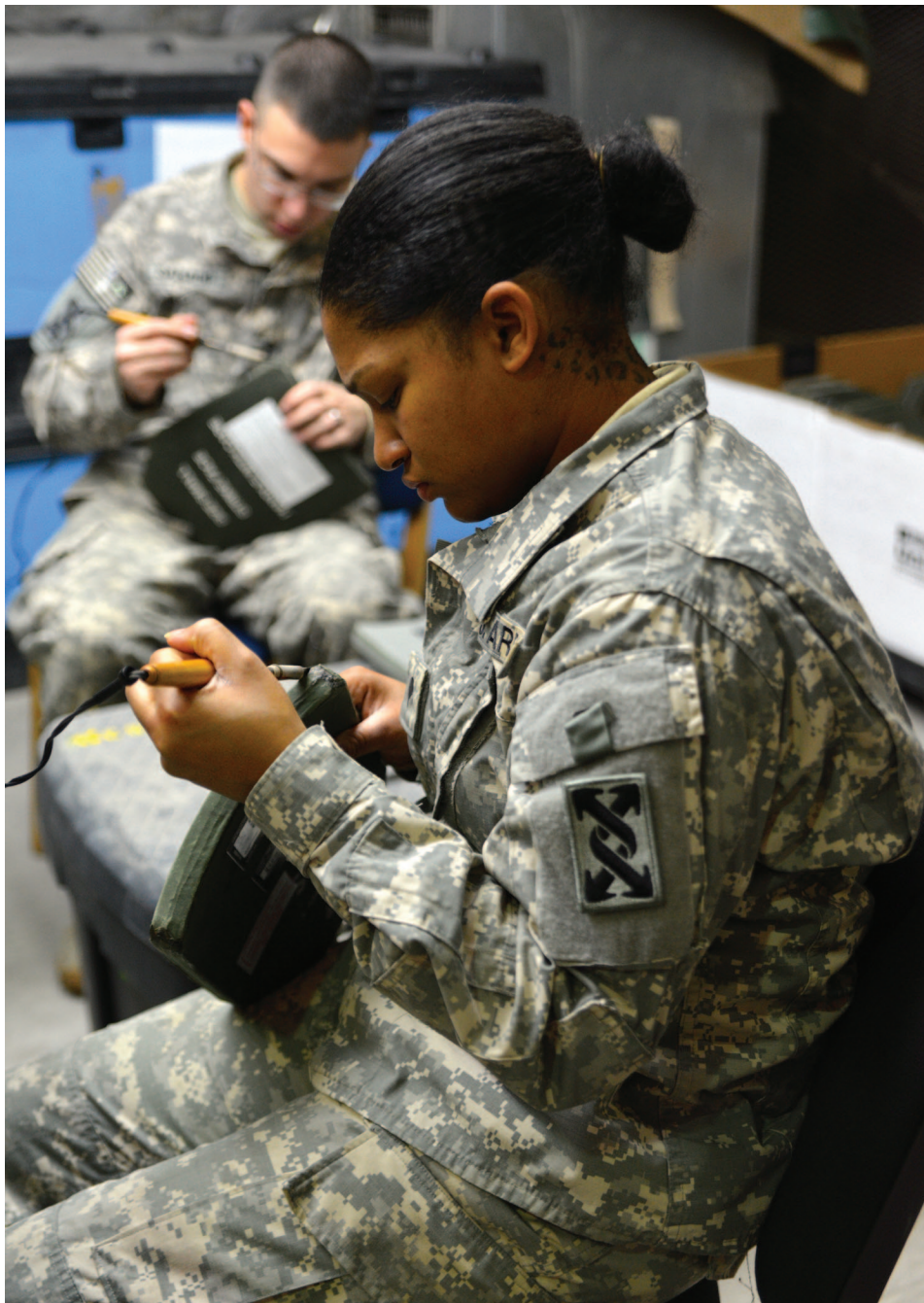
Specialist Chanel Coco (right), support specialist, and Staff Sgt. Anthony Sabato (left), intelligence analyst, 143d ESC, use soldering irons to make repairs to the outer cover of damaged plates Feb. 13 at Transit Center Manas, Kyrgyzstan. The hot soldering irons allow the plate team to melt composite backing over any rips or tears that might expose the plates' interior.
