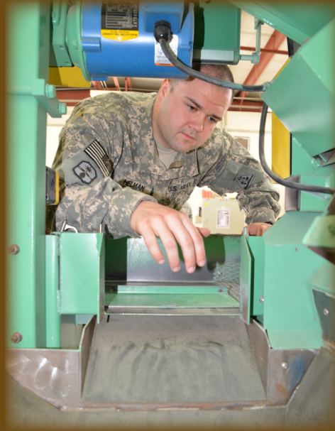
Specialist Zackary T. Helman, an ammunition stock control and accounting specialist with the 371st Sustainment Brigade, inspects an Automated Tactical Ammunition Classification System (ATACS) Jan. 14 at Camp Arifjan, Kuwait. Developed by Cybernet Systems Corporation, the ATACS can inspect and sort up to 5,000 rounds of mixed ammunition in one hour.
