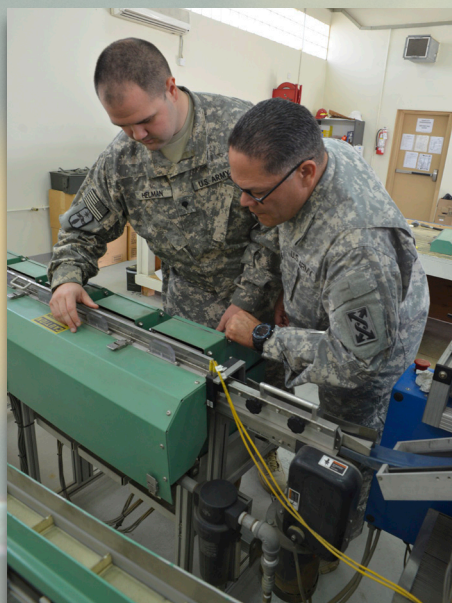
Specialist Zackary T. Helman (left) with the 371st Sustainment Brigade and Sgt. 1st Class Guillermo Matos (right) with the 143d ESC check for dirt and debris in the ATACS at Camp Arifjan, Kuwait. The country's dusty climate makes the machine susceptible to jammed belts and clogged sensors.
