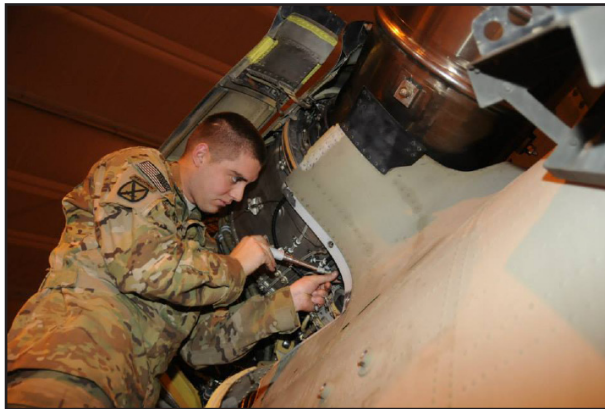
Spc. Travis Shoemaker, an aircraft powerplant repairer with D Company, 3rd Battalion (General Support), Task Force Phoenix, 10th Combat Aviation Brigade, replaces a combustor drain valve gasket on a CH-47 Chinook helicopter Dec. 11, 2013, at Bagram Airfield, Afghanistan. (Photo by Staff Sgt. Todd Pouliot, 10th Combat Aviation Brigade)
