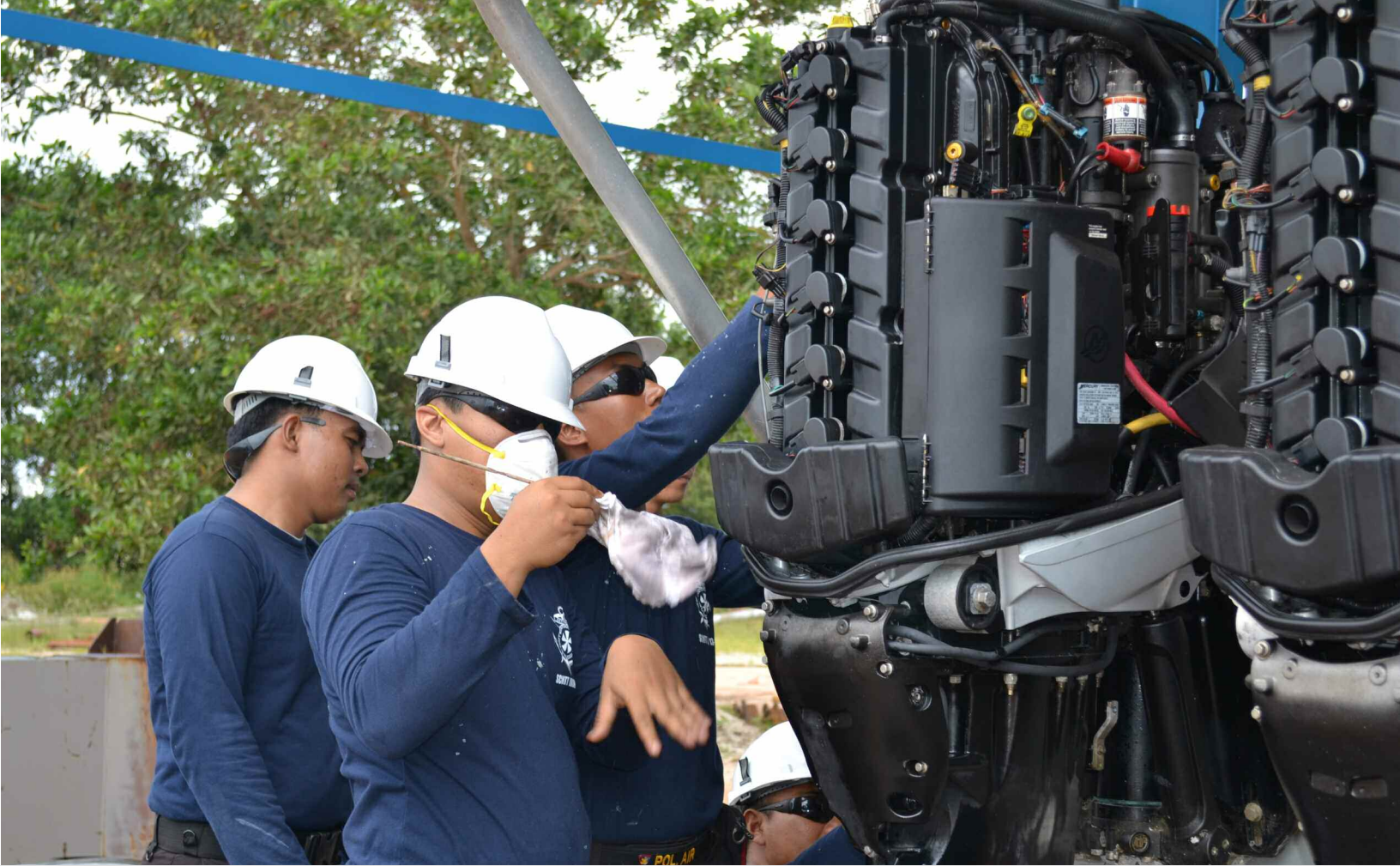
Clearing the coolant passages, a member of the POLAIR performs preventative maintenance on a sophisticated 200+ horse power four cycle marine outboard engine. Below, pre-underway brief. - 24 Feb 2013, Photo LCDR Stephen Bower, USN.
