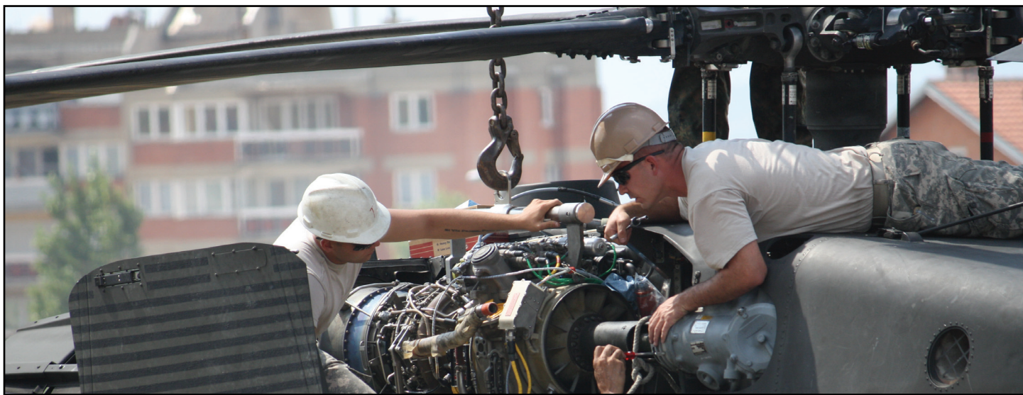
U.S. Army Spc. Nathan Thompson (left) and Sgt. Terry England (right), with Detachment 2, Company B, 638th Aviation Support Battalion, replace the engine on a UH-60 Black Hawk helicopter that made a precautionary landing at Camp Prizren due to an engine fault light Aug. 21. The soldiers were part of a Downed Aircraft Recovery Team that provides a mobile maintenance capability that enables disabled aviation assets a path to return to service. (Photo courtesy of U.S. Army Staff Sgt. Brian Phelps, Det. 2, Co. B, 638th ASB)
