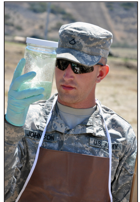
Pfc. Jonathan Johnson, petroleum laboratory specialist with the 316th Quartermaster Battalion out of Okmulgee, Okla., visually inspects a fuel sample for contaminants during a quartermaster liquid logistics exercise at Camp Pendleton.
