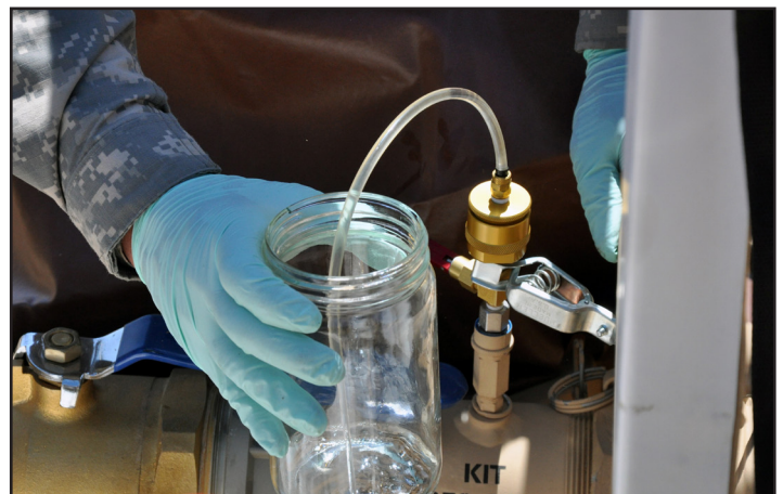
Pfc. Jonathan Johnson, petroleum laboratory specialist with the 316th Quartermaster Battalion out of Okmulgee, Okla., dispenses a fuel sample into a jar during a quartermaster liquid logistics exercise at Camp Pendleton.
