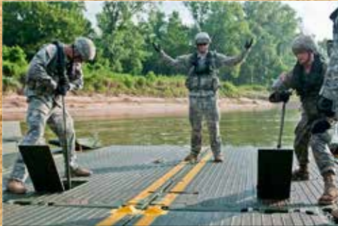
U.S. Soldiers with the 671 st Engineer Company jack up the ramp section of a barge after it leaves port during Operation River Assault at Fort Chaffee, Ark., July 22, 2013. (U.S. Army Reserve photo by Sgt. Dalton Smith, 354 th Mobile Public Affairs Detachment)
