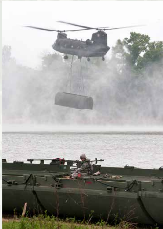
A CH-47 Chinook, piloted by U.S. Soldiers with the 7 th Aviation Battalion, 158 th Aviation Regiment, drops a four-way ramp raft, also known as a six-float and shore to shore full-enclosure floating roadway, into the Arkansas River during a rehearsal for Operation River Assault at Fort Chaffee, Ark., July 22, 2013. (U.S. Army photo by Sgt. Michael T. Crawford/Released)
