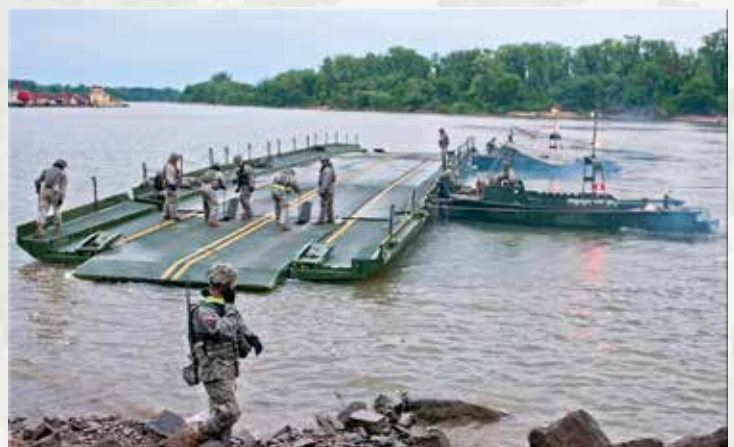
U.S. Army combat engineers with the 671 st Engineer Company (Multi-Role Bridge), 74 th Engineer Company (MRB) and 459 th Engineer Company (MRB), merge bridge sections together to create a barge to transport vehicles across the Arkansas River during Operation River Assault at Fort Chaffee, Ark., July 24, 2013. (U.S. Army photo by Sgt. Dalton Smith/Released)
