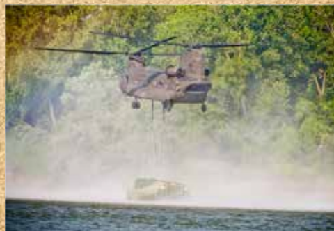
A CH-47 Chinook, piloted by U.S. Soldiers with the 7 th Aviation Battalion, 158 th Aviation Regiment, drops a four-way ramp raft, also known as a six-float and shore to shore full-enclosure floating roadway, onto the Arkansas River during a rehearsal for Operation River Assault at Fort Chaffee, Ark., July 22, 2013. (U.S. Army photo by Sgt. 1 st Class Michel Sauret, 354 th Mobile Public Affairs Detachment)
