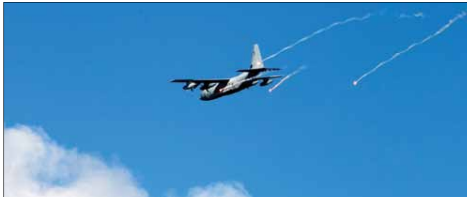
A KC-130J Super Hercules releases flares Aug. 27 above a training island off the coast of Ie Shima. The flares are used to create new heat signature decoys for heat-seeking missiles to follow. The KC-130Js are with Marine Aerial Refueler Transport Squadron 152, Marine Aircraft Group 36, 1st Marine Aircraft Wing, III Marine Expeditionary Force.
