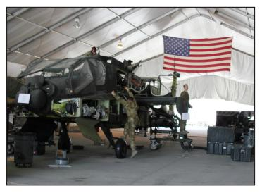
AH-64 Apache helicopter maintenance Soldiers assigned to D Company, 1st Attack/Reconnaissance Battalion, 501st Aviation Regiment, Task Force Dragon, inspect for deficiencies during a 500-hour phase maintenance inspection June 27, at Forward Operating Base Fenty. (Photo by Sgt. Armando Avila, Task Force Dragon)
