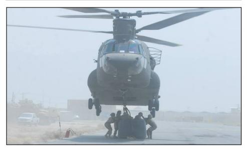
Pfc. Chiquita Albritton, assigned to E Company, 3rd General Support Aviation Battalion, 10th CAB, utilizes a grab hook during sling load training on Bagram Airfield, Afghanistan, July 30. E Co., 3-10 GSAB, conducts sling load training to enhance cargo movement in support of Operation Enduring Freedom. (Photo by Spc. Alexander Naylor, Combat Camera)
