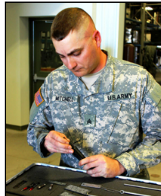
Sgt. Lindley Mitchell, small arms repairer, 245th Maintenance Company, and Carlinville, Ill. resident, gauges an M16A2 weapons system part. Gauging lets Mitchell know if the parts are serviceable and the weapon safe to fire. The 245th MC conducted Extended Combat Training in Ft. Leonard Wood, Mo., May 12-25 to hone their Military Occupational Specialties, conduct driver's training and practice Physical Readiness Training. (U.S. Army Photo by Sgt. 1st Class James Turner, 245th Maintenance Company)
