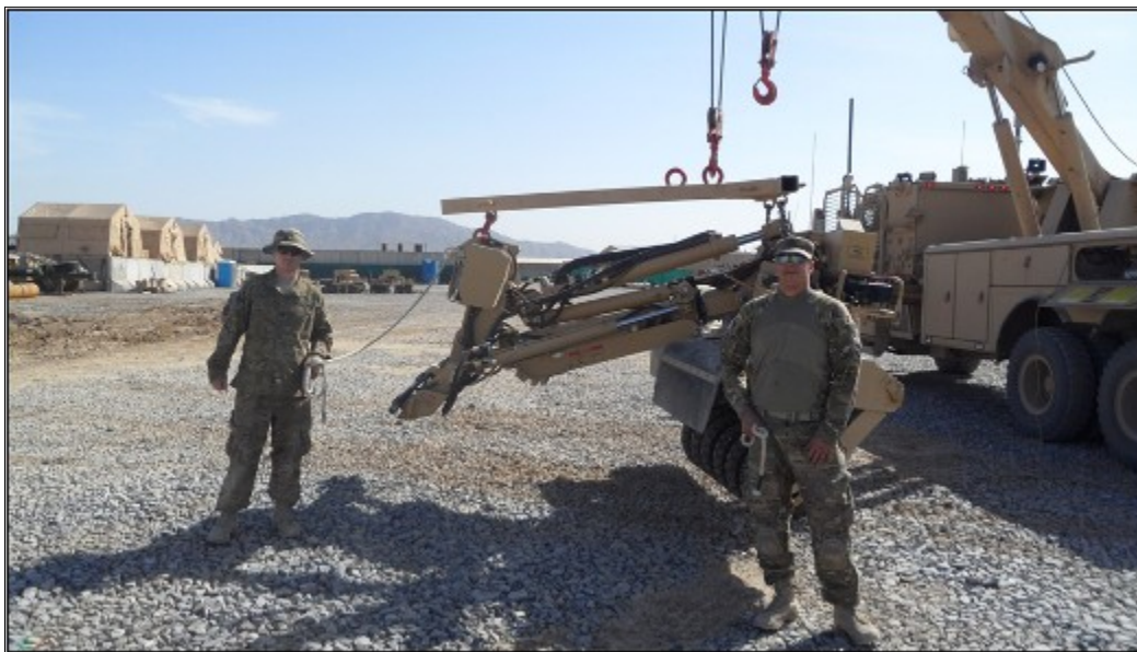
KANDAHAR, Afghanistan – Specialist Nicholas Martindale (left) and Sergeant Jason Newman (right) demonstrate the use of their Mine Roller Sling on a Maxxtow Recovery Vehicle at Forward Operating Base Walton (Photo by U.S. Army Specialist John Hinojosa, 370th Sapper Company Wheeled Vehicle Mechanic)
