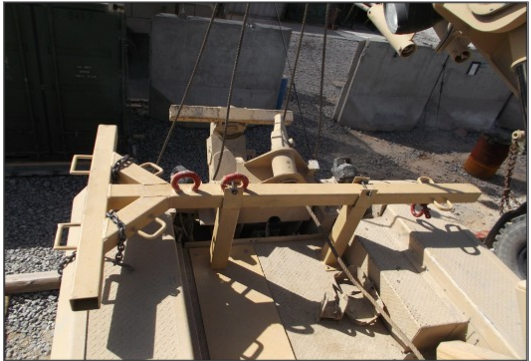
KANDAHAR, Afghanistan – “Don’t Wing It, Sling It” Mine Roller Sling shown in its stowed position on the back of a Maxxtow Recovery Vehicle at Forward Operating Base Walton (Photo by U.S. Army Specialist John Hinojosa, 370th Sapper Company Wheeled Vehicle Mechanic)
