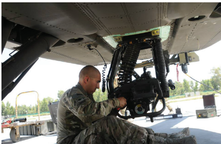
Spc. Edgar Flores, an AH-64 Apache helicopter armament repairer with D Company, 1st Battalion (Attack), 501st Aviation Regiment, Task Force Dragon, installs a 30-millimeter M230 Chain Gun onto an Apache June 18, at Forward Operating Base Jalalabad, in Nangarhar Province, Afghanistan. TF Dragon, an aviation unit from Fort Bliss, Texas, is flying with 10th CAB/TF Falcon in Operation Enduring Freedom XIV. (Photo by Staff Sgt. Todd Pouliot, 10th Combat Aviation Brigade)
