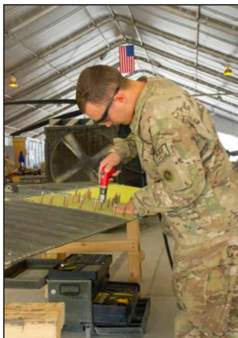
SPC Samuel Miller, from Ahwahnee, Calif. fastens rivets to a helicopter stabilator on Kandahar Airfield, Afghanistan. Miller is a 15G Aviation Structural Repairer with the 1106th Theater Aviation Sustainment Maintenance Group, a California National Guard unit from Fresno, Ca. who is supporting maintenance operations for Task Force Falcon (U.S. Army photo by CPT Chad Ashe)
