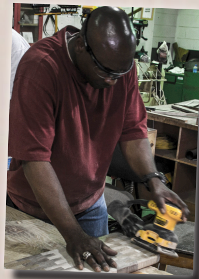
Sgt. Maj. Gilbert Hurte smooths the edges on his cutting board by sanding them down with a power sander.
