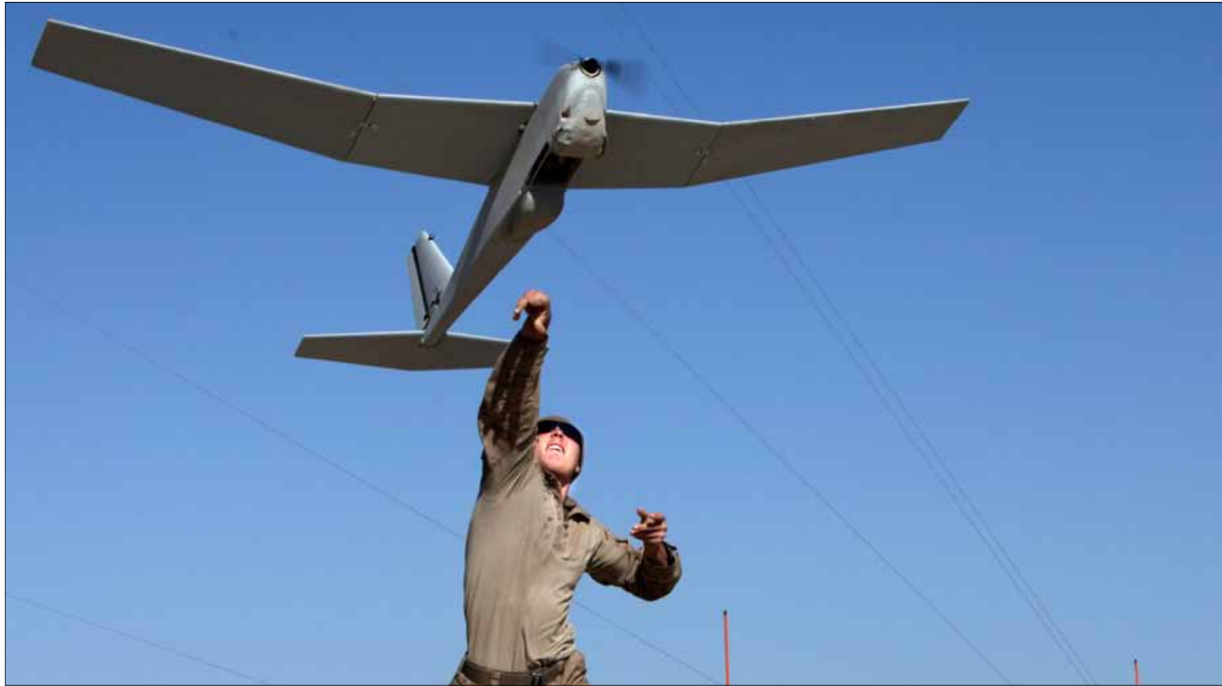
Lance Cpl. Nathan Bush launches the Puma during an operation at Patrol Base Boldak March 4. To operate, the Puma must be launched by hand. Bush is a member of Weapons Company with 2nd Battalion, 7th Marine Regiment. Weapons Company, 2/7, is one of the few Marine Corps units in Helmand province still operating independently of the Afghan National Army and remains focused on counterinsurgency operations.
