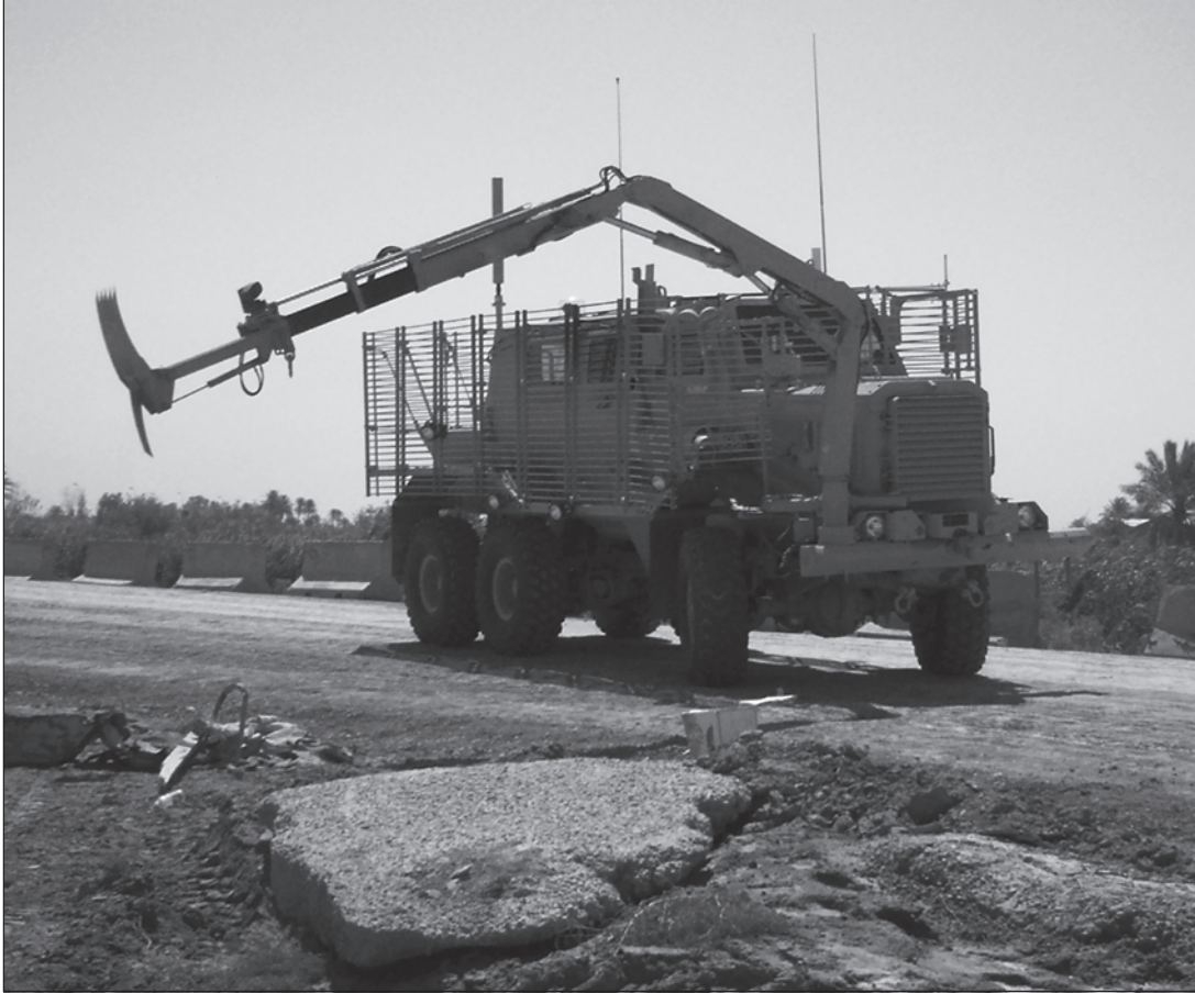
The robotic arm of the Buffalo searches for suspected IEDs.
