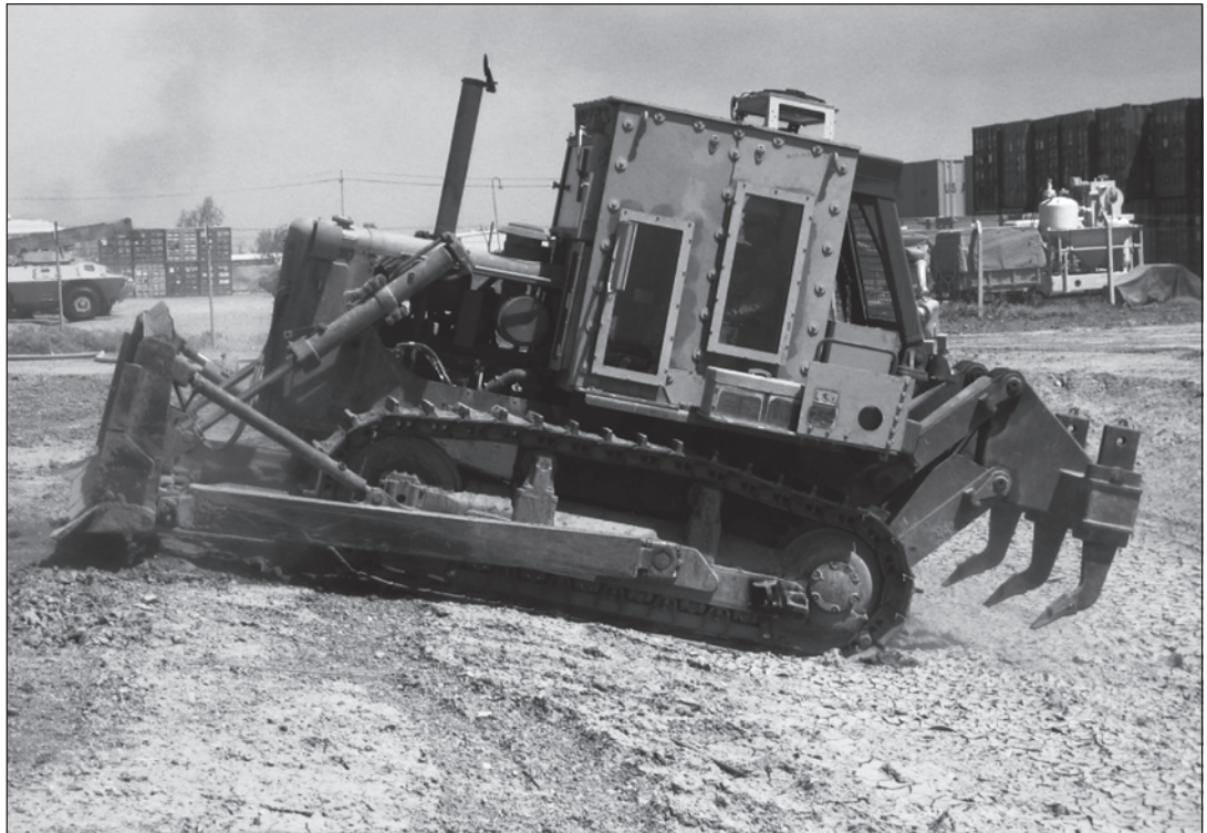
An up-armored D7 dozer is tested.
