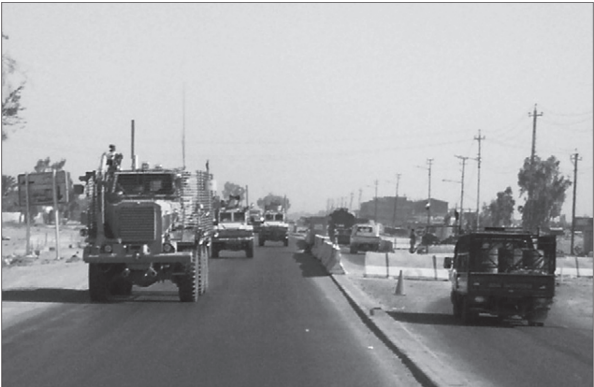
These mine-protected vehicles, the Buffalo and the RG-31, are used in the counter-IED fight.
