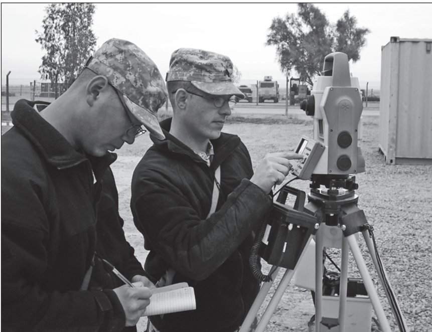
Two survey Soldiers take field notes and set up the Geodimeter 5600.
