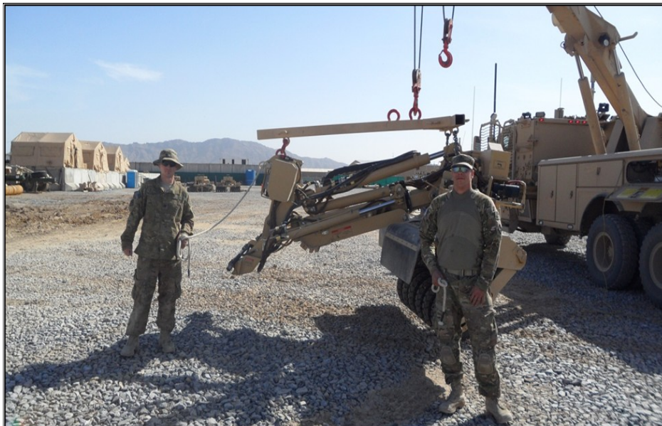
KANDAHAR, Afghanistan – Specialist Nicholas Martindale (left) and Sergeant Jason Newman (right) demonstrate the use of their Mine Roller Sling on a Maxxtow Recovery Vehicle at Forward Operating Base Walton (Photo by U.S. Army Specialist John Hinojosa, 370th Sapper Company Wheeled Vehicle Mechanic)
