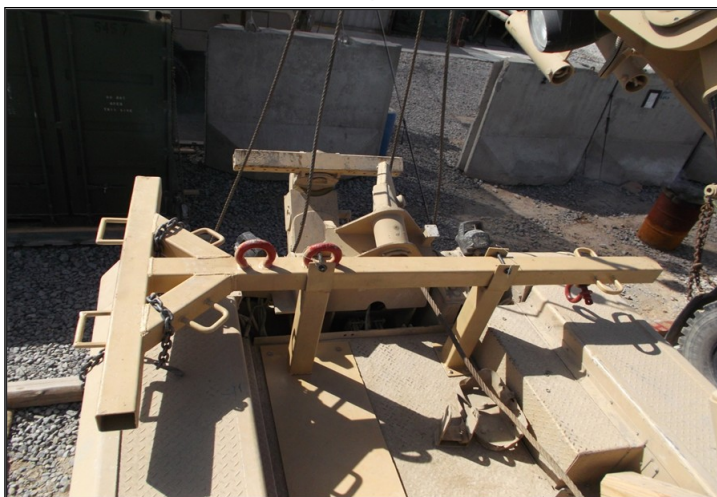
KANDAHAR, Afghanistan – “Don’t Wing It, Sling It” Mine Roller Sling shown in its stowed position on the back of a Maxxtow Recovery Vehicle at Forward Operating Base Walton (Photo by U.S. Army Specialist John Hinojosa, 370th Sapper Company Wheeled Vehicle Mechanic)
