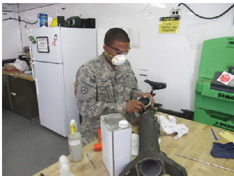
Powertrain Repairer SGT Bianca Allen prepares a UH-60 component for Non-Destructive Inspection (NDI).
