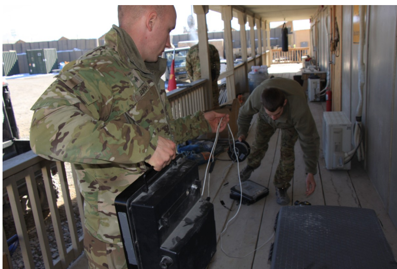
(Above) Explosive Bomb Technicians, Sgt. Christopher Birch and Spc. Cody Hlavka train with an RTR-4 X-Ray scanner to detect contents of unknown packages. This helps the technicians determine the type of threat they are dealing with. (U.S. Army photo by 1 st Lt. Henry Chan, 18 th Combat Sustainment Support Battalion Public Affairs)
